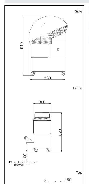
Electric Supply voltage: 220-240 V/1N ph/50 Hz **Electrical power, default:** 0.37 kW Capacity: Maximum kneading (60% hydratation): 8 kg/Cycle Key Information: External dimensions, Width: 300 mm External dimensions, 550 mm Depth: External dimensions, Height: 620 mm **Shipping weight:** 49 kg 10 lt **Bowl capacity:**
